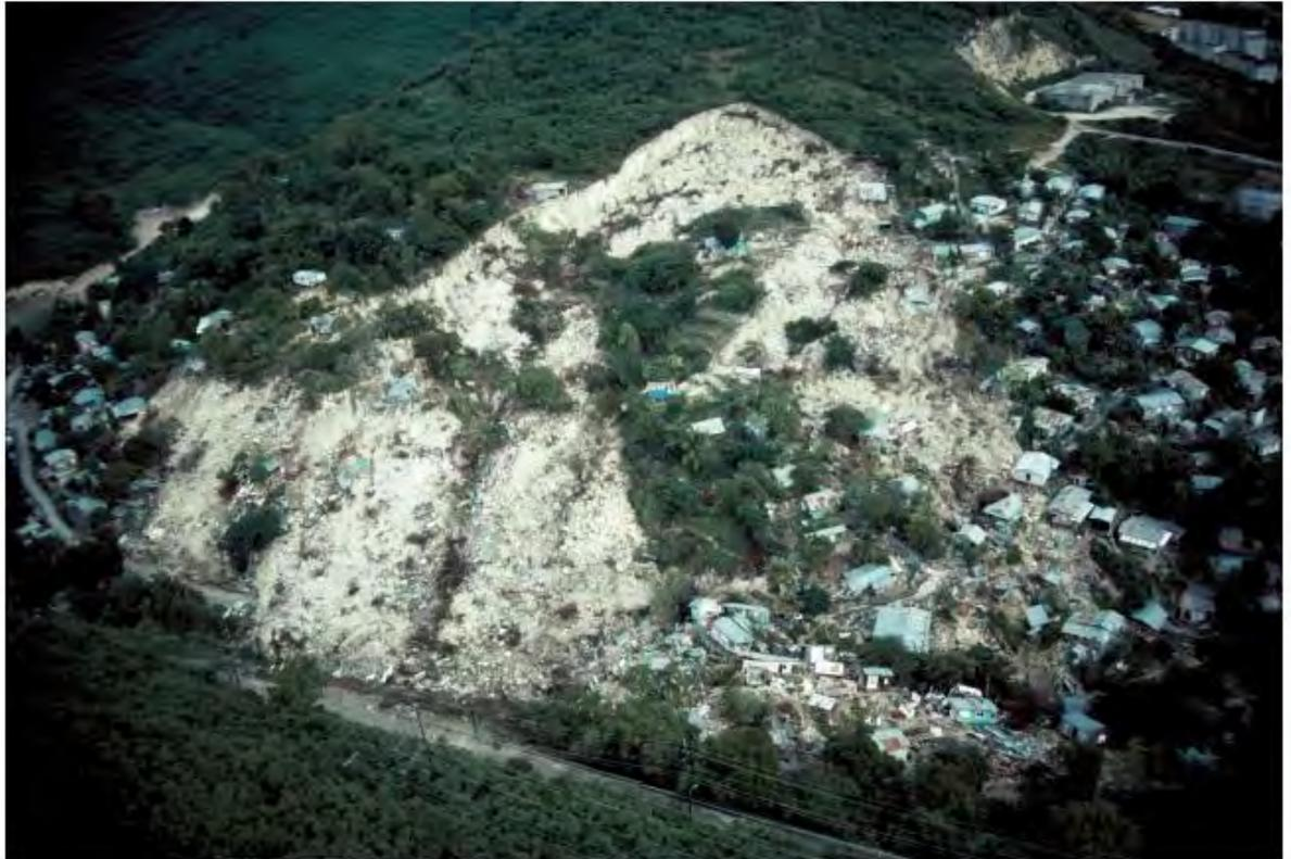
**Figure 26.** The Mameyes, Puerto Rico, landslide, 1985. This landslide destroyed 120 houses and killed at least 129 people. The catastrophic slide was triggered by a tropical storm that produced extremely heavy rainfall. Contributing factors could also have included sewage saturating the ground in the densely populated area, and a leaking water pipe at the top of the landslide. (Photograph by Randall Jibson, U.S. Geological Survey.)
